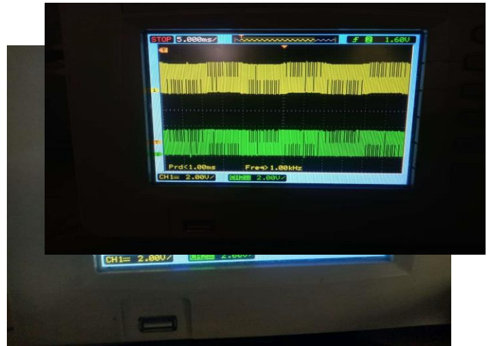
FIG-8.2 SHOWS PWM SIGNAL GENERATED FOR (R+, Y+)
